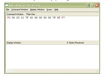
5) Transmit the message to the device by clicking on "Send Sysex" command in "Command Window" menu.
