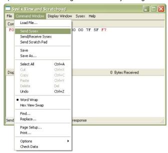
If MIDI-OX is used first time, it is necessary to activate MIDI port to which EDRM-M interface is connected. It must be done for proper data transfer from PC to the interface.
