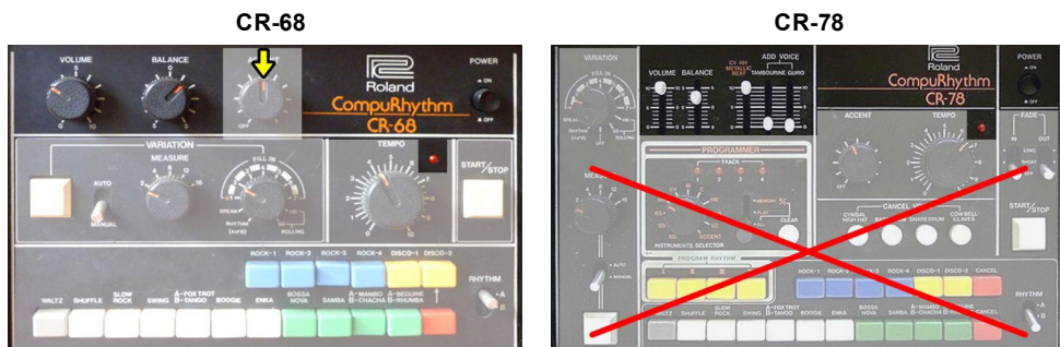
Pic. 4 – Nonfunctional control elements of instrument in "Note" mode
