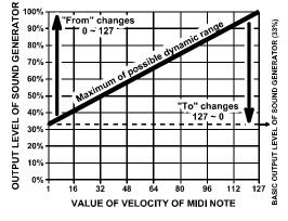
For all others "Velocity" values (from 2 to 126), output level of sound generator is linearly interpolated between minimal and maximal levels (see picture).
