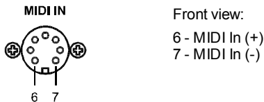
Pic. 3 – Connection of TR-808 to MIDI system
