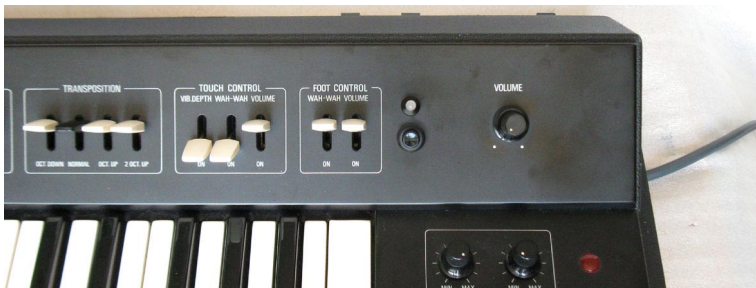
Figure. 4.4 – LED and button installed in SY-2 instrument
