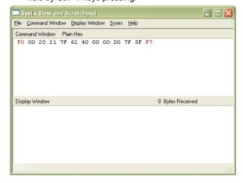
Transmit the message into TR808-M by clicking on "Send Sysex" command in "Command Window" menu.
