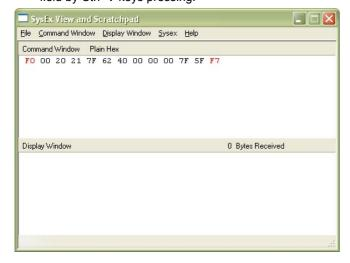
Transmit the message into SH2/9-M by clicking on "Send Sysex" command in "Command Window" menu.
