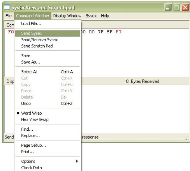
If MIDI-OX is used first time, it is necessary to activate MIDI port to which VS-MIDI interface is connected. It must be done for proper data transfer from PC to the interface.
